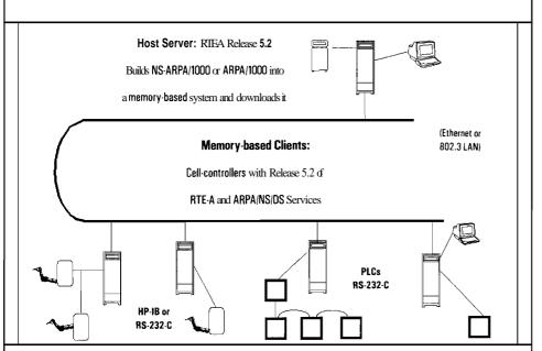
Memory-based systems offer client-server computing to HP 1000 users. The client node is an A-Series memory-based system that is downloaded by a remote host over a LAN. The server node is an A-Series disk-based system that allows users to build the NS-ARPA/1000 (PIN 91790A/R) or ARPA/1000 (PIN 98170A/R) product into a memory-based system, download it, and control it. A single server can download up to 28 clients simultaneously over a LAN.
